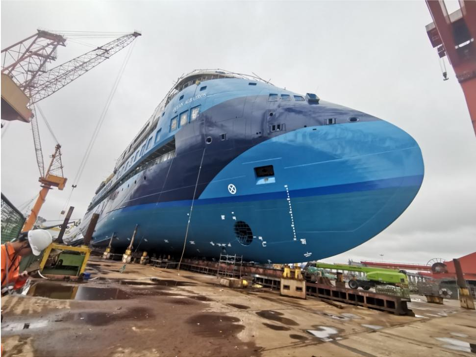
Picture 1: The Ocean Albatros, N.B. CMHI 196-6, sliding to the launching platform.
